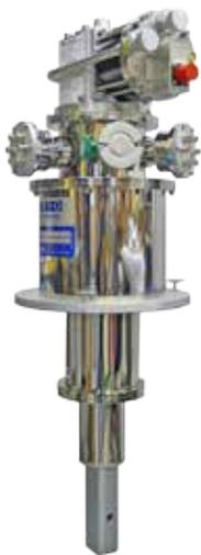
*Custom 4K Sample in Vacuum Refrigerator System with Compact, Rectangular Optical Tail for Electromagnet*
