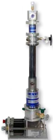
characterization, while model REF-399-D222 (Mossbauer) features low vibration through bellows, spacer and exchange gas isolation. Vibration isolation stand available for Mossbauer and other sensitive experiments.
