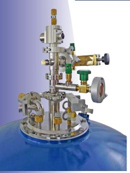
The sample in vapor variable temperature Storage Mount Insert fits into standard storage dewars with 2 inch diameter necks and provide variable temperatures from <1.5 K to 300 K. Samples are cooled by insertion into flowing helium gas exiting from the vaporizer (also known as the diffuser or heat exchanger).
