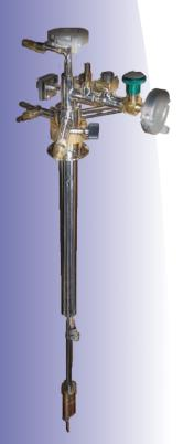
The Variable Temperature Computerized Insert is a top loading sample in vapor variable temperature cryostat. It fits standard 1.4 inch neck diameter (1.5" O.D.) storage dewars, 30, 60 or 100 liters.
