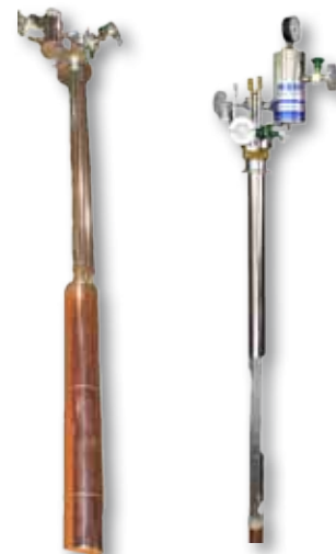
L: HE-3 Top-Loading Sample Insert for ATM R: He-3 PRO Sample in Vacuum
