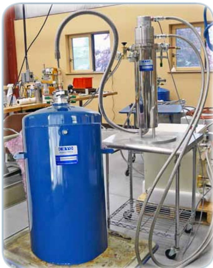
***Cryocool-3-in-1 Unit connected to Optional Liquid Nitrogen Storage Dewar***
