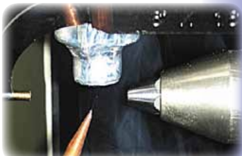
Photo of actual crystal at liquid He temperature with CRYOCOOL system. Photo courtesy of Hakon Hope.
