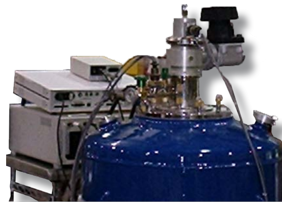
Superconducting Magnet System with 'SuperVariTemp' Magnet Insert
