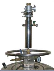
The standard DSTAT SM-2243-DC has a 2.00" sample tube and is very efficient. Cool down losses will depend on the added masses, but should be approximately 0.75 liters of
