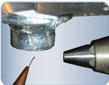
Ice-Free Sample at 8 K using Cryocool-LHe
