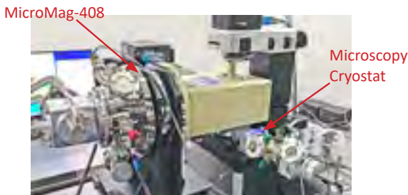
Below: MicroMag-408 installed in end user lab with a Continuous Flow Microscopy Cryostat
