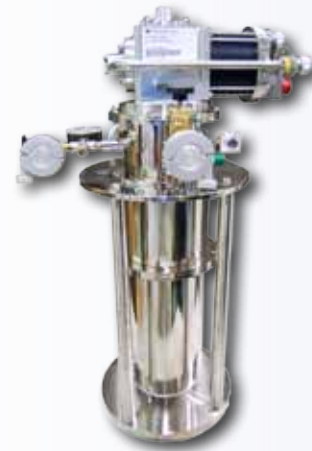
Custom 4 K 1.0 W Sample in Vacuum Tubular Refrigerator System
